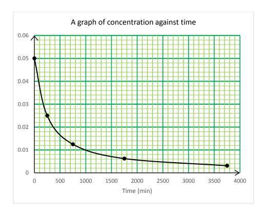
The half-life doubles each time the "initial" concentration is reduced to half its previous value. This behavior indicates a second-order reaction.
