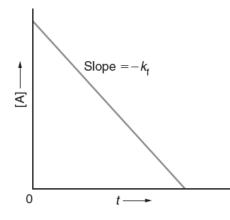
measured time intervals and since volume of sodium thiosulphate gives a measure of amount of iodine remaining in the reaction mixture at given time interval, a graph of volume of thiosulphate versus time is plotted.
