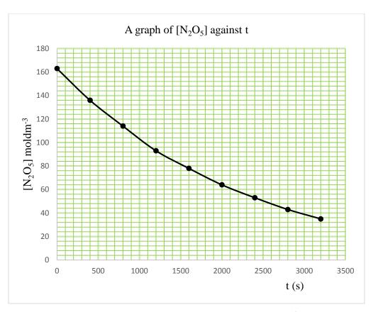
From the graph, Time corresponding to the concentration,  $\frac{163}{2} = 81.5 \text{ moldm}^{-3}$  is the half-life. From the graph, the half-life is 1450s also the successive half-lifes are constant implying that the reaction is first order.
