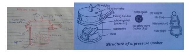
The pressure cooker is a large saucepan made of heavy-gauge aluminum. It has:
