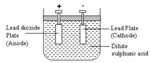
The cathode is lead, the anode is lead dioxide and the electrolyte is dilute sulphuric acid.
