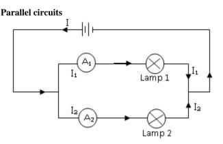
Ammeters are for measuring the current in a parallel circuit. It's characteristic in parallel connections to derive current whenever it reaches the parallel arms of the circuit. But current later recombines to form the original current again before it returns to the cell.
