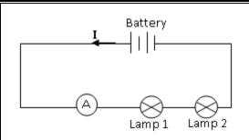
Which is a series connection and current being measured in series.
