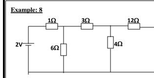
4  $\Omega$  and 12 $\Omega$  resistors are parallel, their effective resistance is  $R_1 = \frac{4 \times 12}{4 + 12} = 3\Omega$
