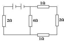
**2.** Eight identical cells each of e.m.f 1.5 and internal resistance  $0.1\Omega$  are connected in a circuit as shown bellow.
