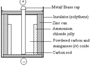
Carbon is the anode and Zinc is the cathode. The electrolyte is ammonium chloride jelly. The chemical reaction between zinc and ammonium chloride is the source of electrical energy is a dry cell and therefore e.m.f is up.
