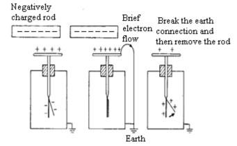
• Bring a negatively charged rod near the cap of the gold leaf electroscope.
