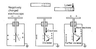
Bring the body under test near the cap of a **charged G.L.E.** If the leaf diverges further, then the body has a charge similar to that on the G.L.E.
