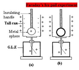
• A metal sphere is suspended by an insulating thread and is given say a positive charge.
