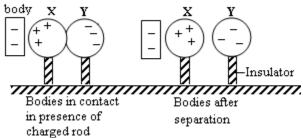
• Support two uncharged bodies, X and Y on an insulated stand and then place them in contact as shown in (a)
