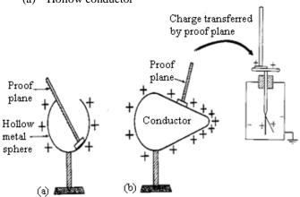
When the proof plane is placed on the outside surface of a charged hollow conductor, charge is transferred to the uncharged G.L.E, the leaf diverges as shown in (a). This proves that charge was present on the outside of the surface.
