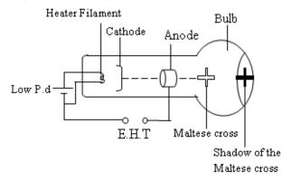
Cathode rays are incident towards the Maltese cross. A shadow of the cross is formed on the fluorescent screen. The formation of the shadow verifies that cathode rays travels in a straight line.
