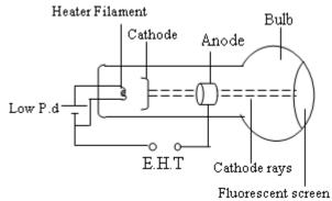
The cathode is heated by a low P.d applied across the filament.
