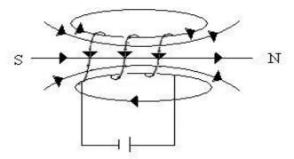
The field pattern due to a solenoid is similar to that of a bar magnet when current is switched on.
