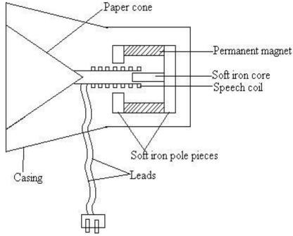
It consists of a light coil of wire known as a speech coil wound tightly round a cylindrical former to which a large thin cardboard cone is rapidly attached. The coil is in a radical magnetic field provided by the permanent magnet which has circular pole.
