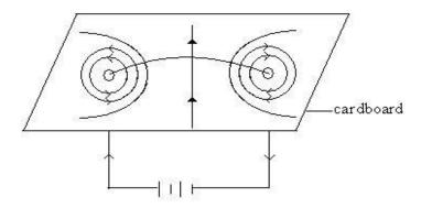
The field lines around each side are concentric circles. At the centre the field lines are straight.
