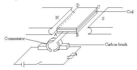
The d.c motor changes electrical energy to mechanical energy. It consists of a rectangular coil which can rotate about a fixed axis in a magnetic field provided by the permanent magnet. The ends of the coil are soldered to two halves of a copper ring (commutator), two carbon brushes press lightly against the commutators
