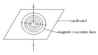
The direction of the magnetic flux depends on the direction of the current in the wire (conductor).
