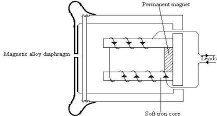
When the phone is lifted, a steady current flows through the solenoids. However when a person speaks into the microphone on the other end, the sound energy he makes is converted into varying electrical energy of the same frequency as the original sound.
