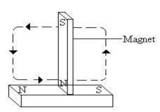
In this method, the steel bar is stroked from end to end several times in one direction with one pole of a magnet.
