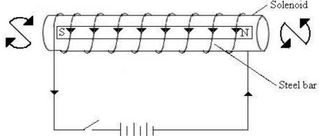
The material to be magnetized is inserted into a solenoid to which a steady d.c is flowing. The current is switched on for a short time.
