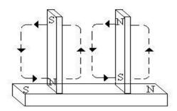
In this method, the steel bar is stroked from the centre outwardly with unlike poles of the two magnets. The polarity produced at the end of the bar is also of the opposite kind to that of the stroking pole.
