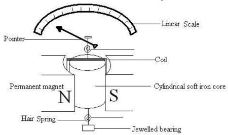
It consists of a rectangular coil with many insulated turns wound on an aluminum fomer, soft iron cylindrical core between the curved poles of a powerful permanent magnet, the springs which control the rotation of the coil, a pointer and a linear scale. The current is led in and out by two hair springs.
