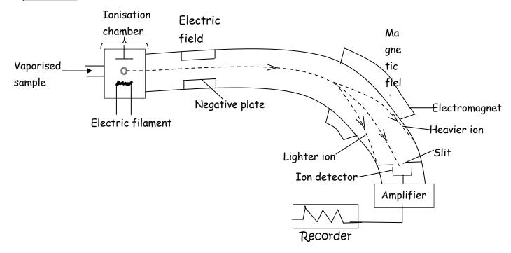
The mass spectrum is evacuated and the sample is vapourised by heating.
