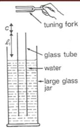
C = End correction,  $l_1$ ,  $l_2$  = Length of air column.
