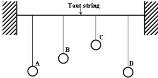
Hang four pendulum bobs on the same taut string such that pendulum, A has variable length while B, C and D have different fixed lengths.
