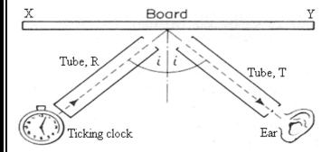
XY is a hard plane surface, R is a closed tube and T is an Open tube.
