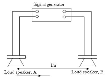
Two loud speakers A and B are connected to the same signal generator so that sound waves from each are in phase and are of the same frequency. Interference of waves from A and B occurs
