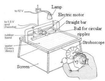
A ripple tank is an instrument used to study water wave properties. It is a shallow glass trough which is transparent. The images of the wave are projected on the screen which is placed below it.
